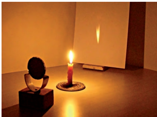
Fig. 11.15 Real images formed by a concave mirror
