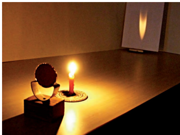
Fig. 11.15 Real images formed by a concave mirror
