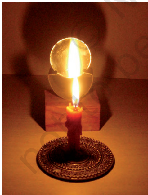
Fig. 11.16 Virtual image formed by a concave mirror
