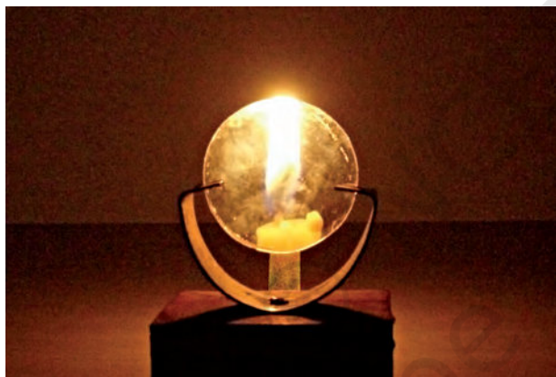
Fig. 11.26 Virtual image formed by the convex lens
